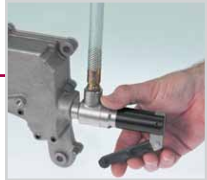
3 Releasing the lever expands the collets for a safe secure leak free connection
