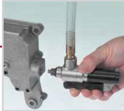
2 Insert into the threaded port
